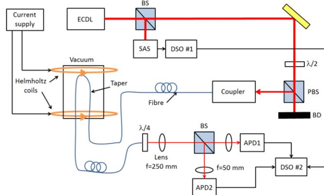
Fig. 1 (Color online) Schematic of experimental setup. ECDL: extended cavity diode laser, BS: beam splitter, SAS: saturated absorption spectroscopy, DSO: digital storage oscilloscope, PBS: polarizing beam splitter, BD: beam dump, APD: avalanche photodiode.
