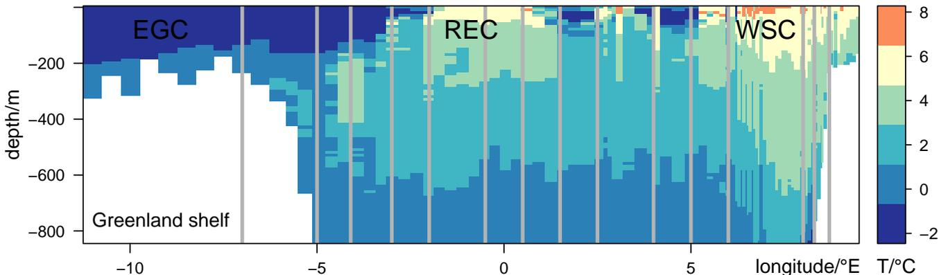
FIG. 2: Temperature field of the upper 800 m of Fram Strait at a latitude of  $78^{\circ}50'N$ . The data was acquired during a cruise with RV Polastern between June 24th and July 11th, 2011. White areas correspond to sea floor. The bold perpendicular lines symbolize the longitudes of the mooring lines, a degree longitude corresponds to roughly 20 km here.
