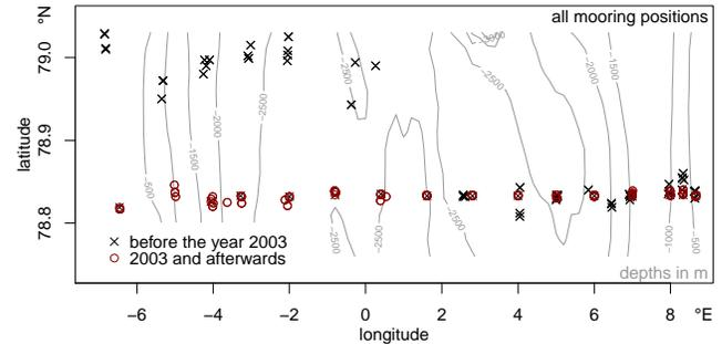
FIG. 1: Map of the mooring positions in Fram Strait. The meridional distance between  $78.8^{\circ}$  N and  $79^{\circ}$  N is around 20 km which is the same as the zonal spacing. For our analysis only the measurements from 2003 and afterward ( $\circ$ ) are taken.
