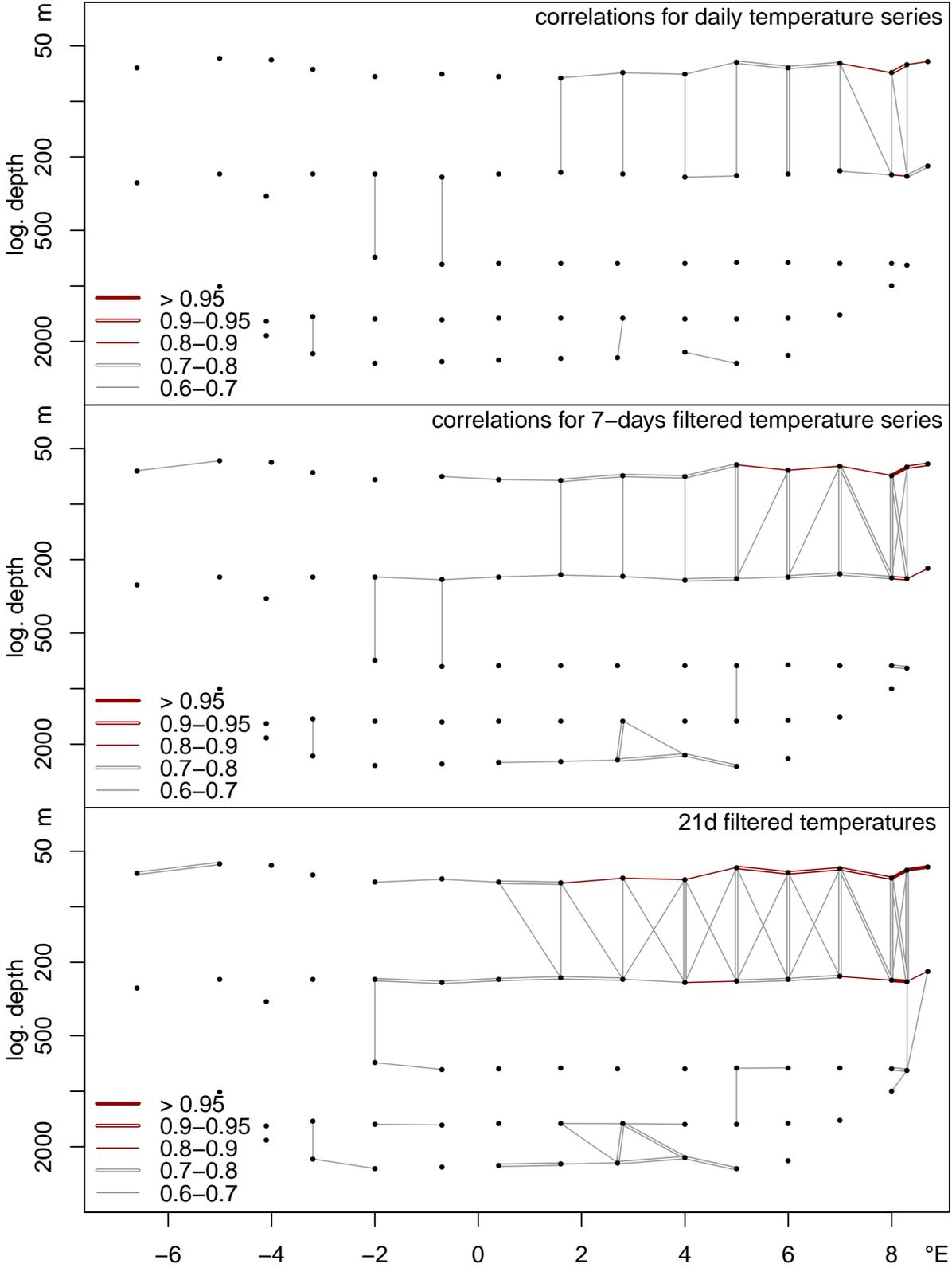
FIG. 3: Temperature correlations coefficients between nearest and 2nd nearest neighbors of all timeseries since 2003 for daily means (top) and with a 7-day filter (bottom). The bullets represent the average instrument position (depth and longitude), for this reason the mooring lines are not straight as sketched in Fig.2.
