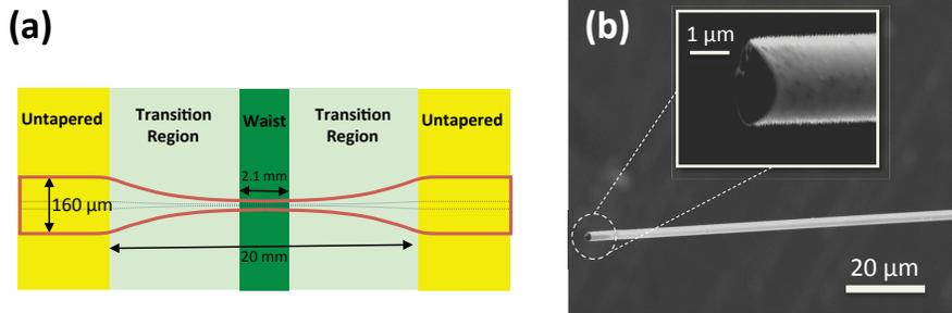
Figure 4: (a) Schematic profile of the tapered fiber; the length of the untapered fiber is  $\sim 18 \text{ mm}$  on each side; the schematic is not to scale. (b) SEM images of the tapered fiber broken at the waist.
