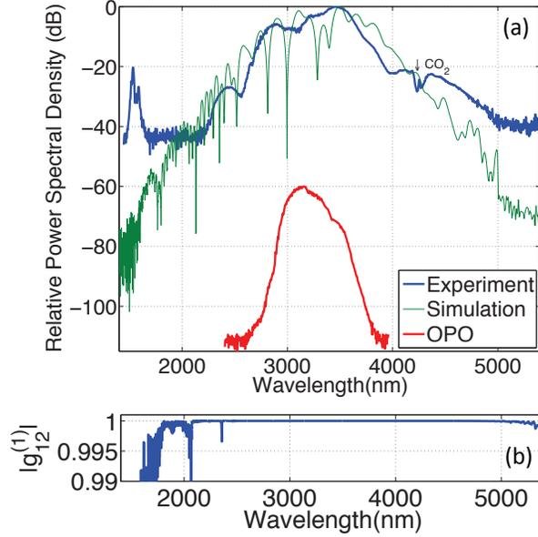
Figure 5: (a) Spectrum of the OPO output broadened by the tapered  $\text{As}_2\text{S}_3$  fiber compared with the simulation result (the OPO spectrum is intentionally shifted), (b) calculated degree of coherence,  $g_{12}^{(1)}$  as defined in [19].
