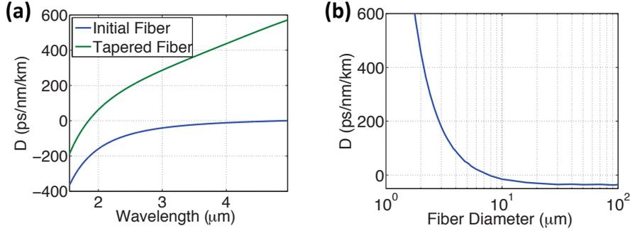
Figure 1: (a) GVD parameter of the initial fiber, a step index  $\text{As}_2\text{S}_3$  fiber with core and cladding diameter of  $7 \mu\text{m}$  and  $160 \mu\text{m}$ , respectively, and an NA of 0.2, compared with that of the fundamental mode of a tapered fiber with diameter of  $2.3 \mu\text{m}$ , (b) GVD parameter of the fundamental mode of the tapered fiber at  $3.1 \mu\text{m}$  as a function of the fiber diameter.
