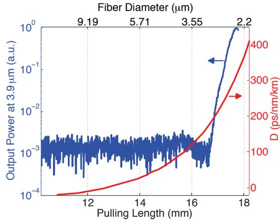
Figure 3: The output power at  $3.9 \mu\text{m}$  during the tapering process (blue curve) versus the pulling length (bottom axis) and corresponding diameter of the fiber waist (top axis), and the calculated GVD parameter of the fundamental mode in the taper waist (red curve).
