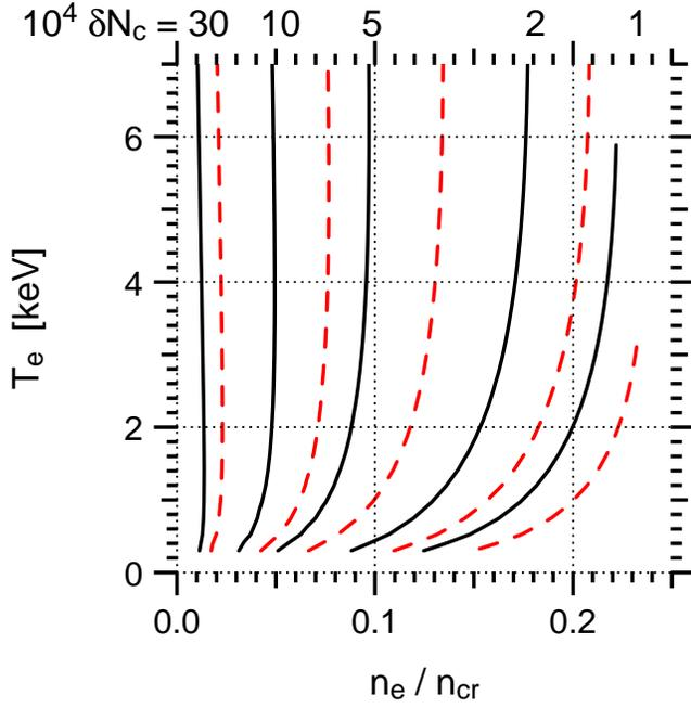
FIG. 10. (Color online.) Threshold Langmuir wave amplitude for collisions,  $\delta N_c$ . LW  $\omega_2$  and  $k_2$  are for phase-matched SRBS with a natural LW (black solid curves of Fig. 7), and pump wavelength  $\lambda_0 = 351$  nm. Black solid:  $Z_{\text{eff}}=1$ . Red dash:  $Z_{\text{eff}}=4$ . From right to left, curves are for  $\delta N_c = [1, 2, 5, 10, 30] \times 10^{-4}$ .
