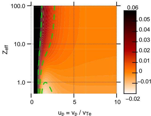
FIG. 6. (Color online.) Relative error  $\epsilon = 1 - \hat{t}_{\text{appr}}/\hat{t}_{\text{ex}}$  between the exact and approximate results from Eqs. (29,30), respectively, for collisional  $\hat{t}$ ; see text for details. The green curves are  $\epsilon = [-0.01, 0.01, 0.05]$ .
