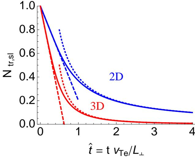
FIG. 1. (Color online.) Trapped electron fraction  $N_{\text{tr,sl}}$  due to transverse side loss for a 2D plane (blue) and 3D cylinder (red) region. The dashed curves are the appropriate early and late time limits. See Eqs. (6) through (12).
