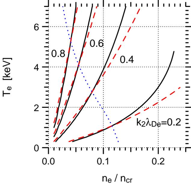
FIG. 8. (Color online.) Langmuir wave  $k_2\lambda_{De}$  phase-matched for SRBS with different  $\lambda_1$  choices, for a pump wavelength  $\lambda_0 = 351$  nm. Black solid:  $\lambda_1$  phase-matched with a natural Langmuir wave, as in black solid curves of Fig. 7. Red dash:  $\lambda_1 = 550$  nm ( $\omega$ 's fixed,  $k$ 's vary). Blue dot:  $\lambda_1 = 550$  nm black-solid contour from Fig. 7.
