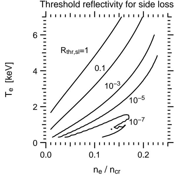
FIG. 14. Threshold reflectivity  $R_{thr,sl} \propto 1/I_0^2$  from Eq. (41) to overcome side loss for  $I_0 = 10^{15}$  W/cm<sup>2</sup>.
