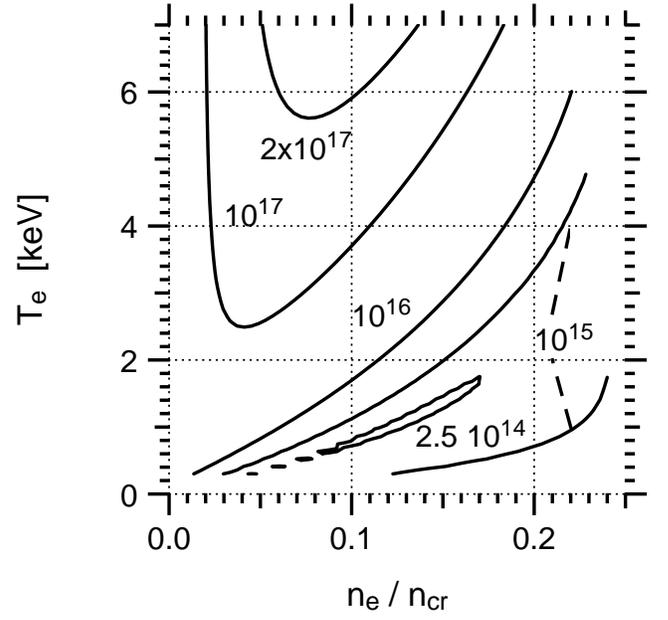
FIG. 13. Critical intensity  $I_{cr}$  from Eq. (40) in W/cm<sup>2</sup> relating laser intensity  $I_0$  and reflectivity  $R$  to LW amplitude:  $\delta N = (I_0/I_{cr})R^{1/2}$ .
