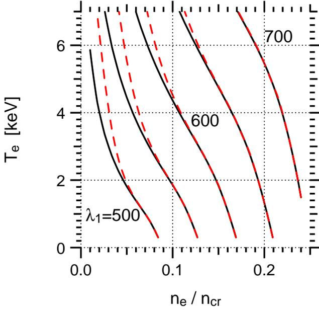
FIG. 7. (Color online.) Wavelength  $\lambda_1$  in nm for SRBS light (increments of 50 nm), for a pump wavelength  $\lambda_0 = 351$  nm. Black solid:  $\lambda_1$  phase-matched with a natural Langmuir wave, satisfying the dispersion relation Eq. (36) with  $\nu_K = 0$ . Red dash:  $\lambda_1$  for the maximum local SRBS spatial gain rate.
