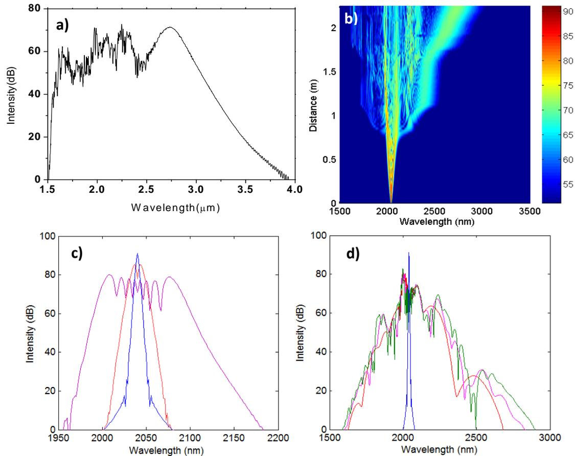
Fig.2: a) Simulated supercontinuum spectra from a 2.25 m length of the designed LMA fiber; b) evolution of the short pulse propagation along the fiber length; c) pulse broadening due to SPM during the initial stage at three different lengths of 25 mm (blue), 125 mm and 650 mm, respectively) of pulse propagation; d) pulse spectra to visualize the broadening of the pulse mainly due to solitons fission at 0.85 m (red), 0.9 m and 0.95 m (green).
