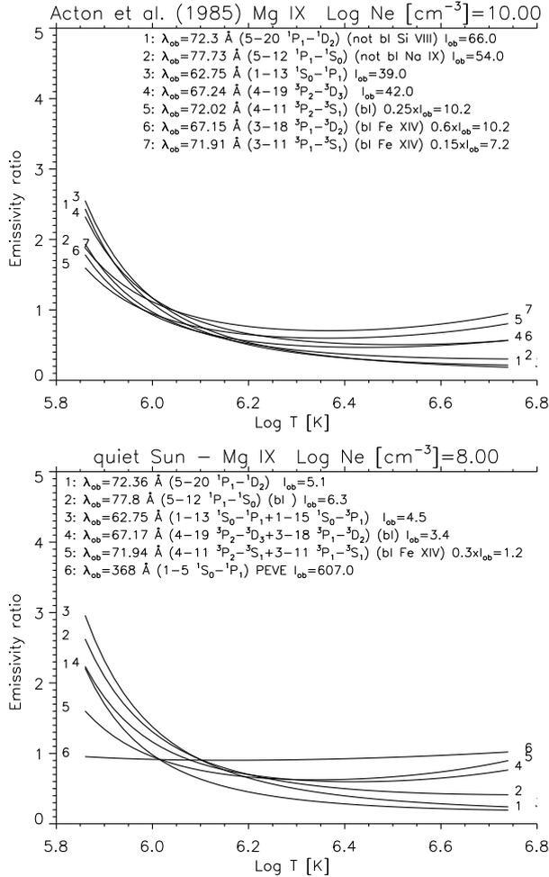
**Fig. 2.** Emissivity ratio curves relative to the main Mg ix lines and the solar flare (A85) and quiet Sun (M72, PEVE) observations.  $\lambda_{\text{ob}}$  indicates the observed wavelength ( $\text{\AA}$ ),  $I_{\text{ob}}$  indicates the observed intensity, sometimes reduced by the amount indicated. (bl) indicates the presence of a blend.
