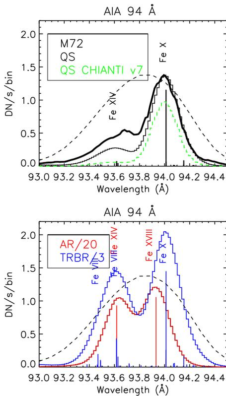
**Fig. 14.** SDO AIA 94 Å simulated count rates, obtained for the quiet Sun (QS), an active region core (AR, reduced by a factor of 20) and a loop base (TRBR, reduced by a factor of 3). The M72 quiet Sun spectrum (normalised) is also shown, as well as the quiet Sun spectrum obtained from CHIANTI v7. The AIA effective area (normalised) is shown as a dash line.
