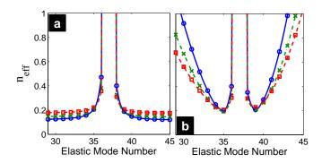
FIG. 4. (Color online) Effective phonon number of the CoM mode (a) and of the elastic mode (b), as a function of the elastic mode frequency for three different photon absorption rate values:  $\kappa_2 = 0$  (blue circle),  $\kappa_2 = 0.5\kappa_1$  (green cross), and  $\kappa_2 = \kappa_1$  (red square). The detuning is set to  $\Delta_c = \omega_m$  and  $\chi \simeq 0.03$ . Laser power is  $\mathcal{P} = 15$  mW and  $\kappa_1 = 0.05\omega_m$ .
