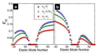
FIG. 7. (Color online) Logarithmic negativity of CoM mode– cavity mode (a), and elastic mode–cavity mode (b) bipartite subsystems as a function of the elastic mode frequency. The detuning is set to  $\Delta_{\rm c} = 0.87\omega_{\rm m}$  and  $\chi \simeq 0.03$ . Laser power is  $\mathcal{P} = 100$  mW and  $\kappa_1 = 0.25\omega_{\rm m}$ .
