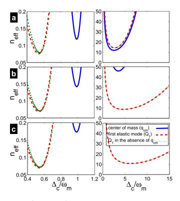
FIG. 2. (Color online) Effective phonon number versus cavity detuning in the good cavity limit  $\kappa_1 = 0.05\omega_{\rm m}$  (left panels) and in the bad cavity limit  $\kappa_1 = 5\omega_{\rm m}$  (right panels): (a)  $\kappa_2 = 0$ , (b)  $\kappa_2 = 0.5\kappa_1$ , and (c)  $\kappa_2 = \kappa_1$ . The elastic mode frequency is  $\Omega_1 \simeq 0.54\omega_{\rm m}$ ,  $\tau_{\rm th} = \Omega_1^{-1}$ , and  $\chi \simeq 0.13$ . Power of the laser is  $\mathcal{P} = 15$  mW.
