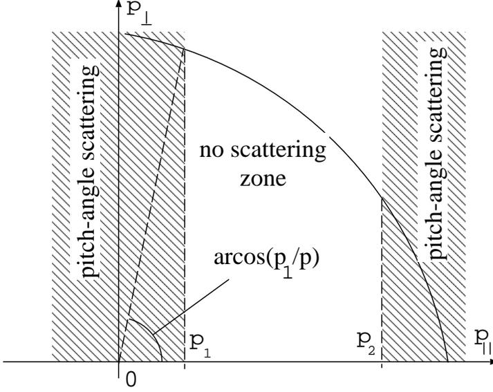
Figure 1: **Momentum space of accelerated protons.** Particle scattering zones on the  $(p_{\parallel}, p_{\perp})$ - plane of momentum space. Protons in the stripes  $p_1 < |p_{\parallel}| < p_2$  are not scattered by waves (see text). Therefore, particles from the domains  $|p_{\parallel}| > p_2$  maintain their propagation direction and promptly escape from the dense gas region.
