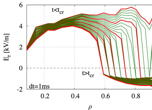
FIG. 4: (Color online) Radial electric field profile for representative times. Lines are separated by 1 ms and thick lines by 5 ms. The starting ( $t < t_{cr}$ )  $E_r(\rho)$  is positive.
