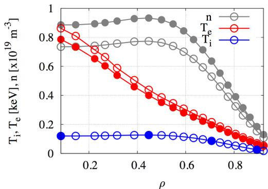
FIG. 1: (Color online) Plasma radial profiles for selected times: low (high)  $n$  in open (closed) circles. The evolution is given through  $\frac{1}{n} \frac{\partial n}{\partial t} = 3 \text{ s}^{-1}$ ,  $\frac{1}{T_e} \frac{\partial T_e}{\partial t} = -1.5 \text{ s}^{-1}$ , and  $\frac{\partial T_i}{\partial t} = 0$ .
