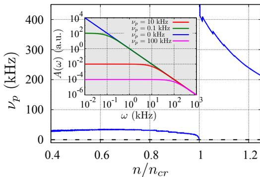
FIG. 5: (Color online) Density dependence of the neoclassical poloidal viscosity during the transition.  $n_{cr}$  is locally defined as the  $n$  at which  $E_r$  passes through 0 (inset: frequency dependence of the neoclassical damping for several values of  $\mu_p$ ).
