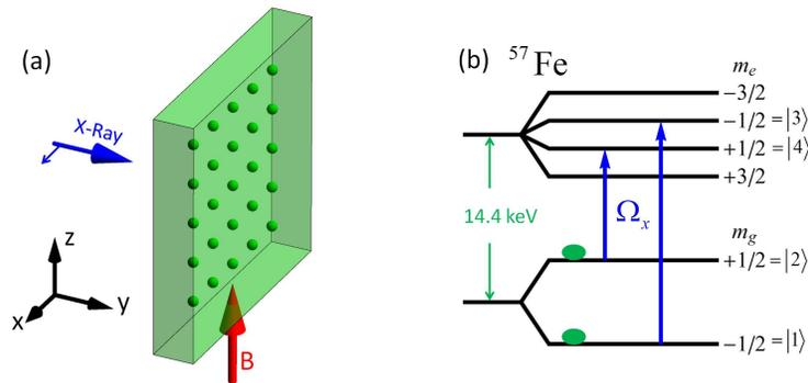
FIG. 1: (a) Nuclear forward scattering setup. The blue arrow depicts the linear polarized x-ray pulse propagating in  $y$  direction and  $\mathbf{B}$  is the external magnetic field initially parallel to the  $z$ -axis. (b) Hyperfine level structure of  $^{57}\text{Fe}$ . The blue solid arrows denote the  $\Delta m = m_e - m_g = 0$  transitions driven by the x-ray pulse which is linearly polarized in the  $x$  direction.
