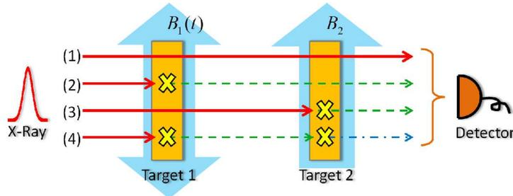
FIG. 5: The setup of magnetically induced nuclear exciton echo with two targets. The orange rectangles depict the targets, and the red pulse the input x-ray. Yellow crosses illustrate the formation of the nuclear exciton. The light blue up-down thick arrows show the applied magnetic fields: the dynamical  $\mathbf{B}_1(t)$  is applied to target 1, whereas the static  $\mathbf{B}_2$  is applied to target 2. (1)(2)(3)(4) are four possible coherent scattering channels (see text for details).
