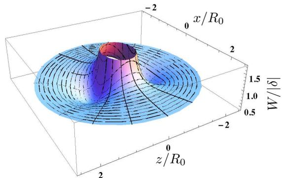
FIG. 3. (Color online) Potential of the  $\theta = 0$  well state in the  $x$ - $z$  plane for  $\delta > 0$ . Two pronounced minima occur on the  $\pm z$  axes. The potential is azimuthally symmetric around the  $z$  axis.
