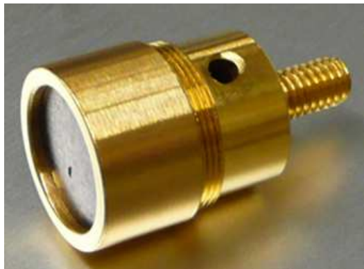
Figure 8. Solid ^{83}\text{Rb}/^{83\text{m}}\text{Kr} source. Left: Photograph of the platinum-implanted ^{83}\text{Rb}/^{83\text{m}}\text{Kr} source. Right: Decay scheme of ^{83}\text{Rb} .
