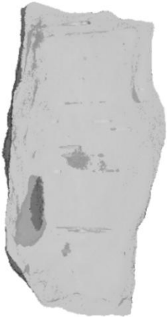
Fig. 9. Tomography of the dry tile at 0°.
