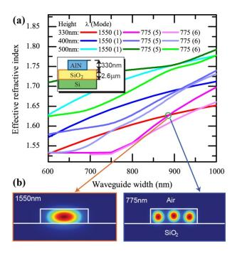
Fig. 1. (a) The calculated dispersion relations for optical modes at 775nm and 1550nm for various film thicknesses. Phase matching between higher order modes at 775nm and 1550nm can be achieved when the waveguide width is adjusted accordingly. In our case the phase-matching condition is fulfilled between the fifth-order mode at 775nm and the fundamental mode at 1550nm (the modal profiles are illustrated in (b)).
