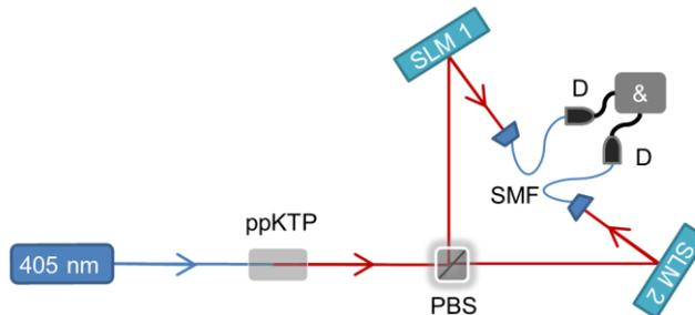
Figure 2: Schematic sketch of the experimental setup. We pump a 5mm nonlinear ppKTP crystal with a 405nm 60mW single-mode diode laser, and obtain 810nm down-converted
