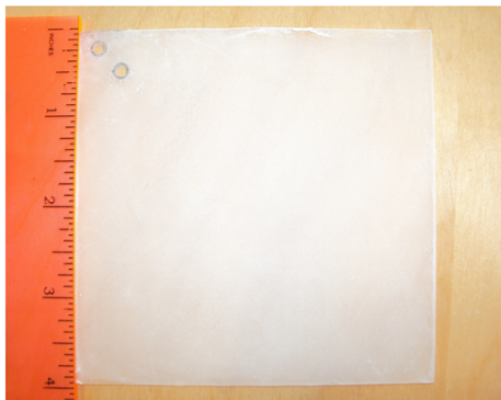
Figure 1. A typical plate used for our studies. The acrylic plate is clear, and the TPB coating has a milky appearance. Two holes were drilled into the plate for attachment to our testing apparatus (Figure 2).
