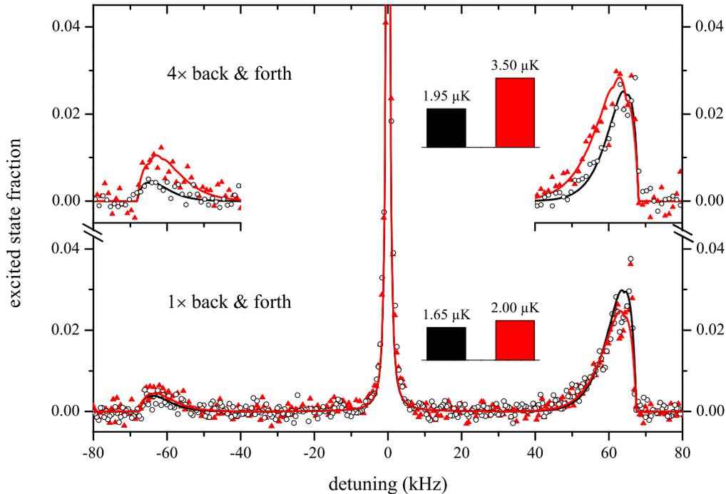
**Figure 3.** Sideband spectra after transporting the atoms once (main graph) and four times (insets) back and forth for 50 mm (solid red triangles) and after holding the atoms in the static lattice for the same time (open black circles). The solid curves are combinations of fits to the carrier and the sidebands, the latter according to [28].
