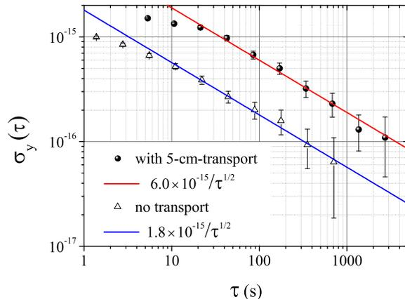
**Figure 6.** Instability with (dots) and without (triangles) transport. In each measurement an interleaved stabilisation scheme is used, in which the clock laser is stabilised in two independent but interleaved stabilisations to the clock transition.
