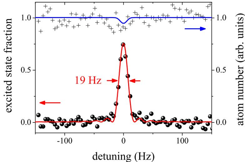
**Figure 5.** Interrogation of the atoms, transported by 5 cm: high resolution spectrum of the clock transition (dots), total atom number (crosses) and calculated losses due to  $^3\text{P}_0 - ^3\text{P}_0$  collisions on the way back (blue line).
