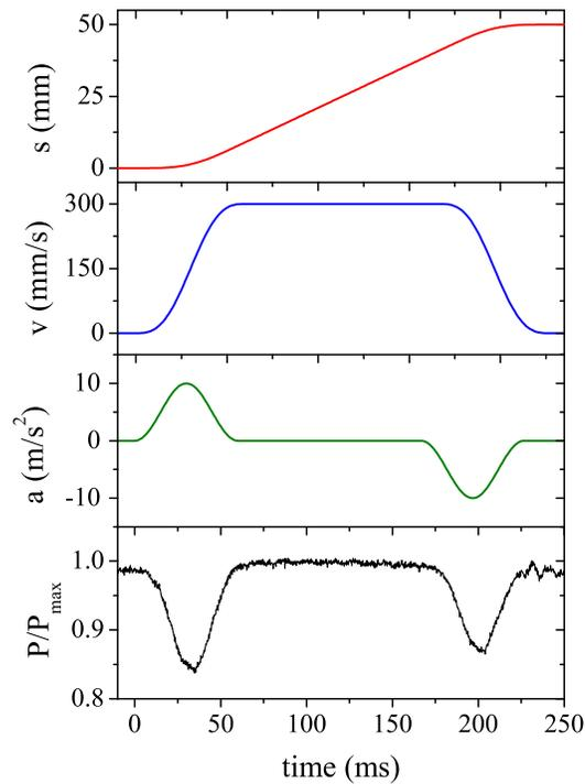
**Figure 2.** Moving lattice trajectory to exhaust the capability of the air bearing translation stages and minimize jerks by a sinusoidal acceleration profile. A 50-mm-transport is completed in 230 ms. From top to bottom position, velocity, acceleration, and the normalized signal of the retro-reflected lattice light are shown.
