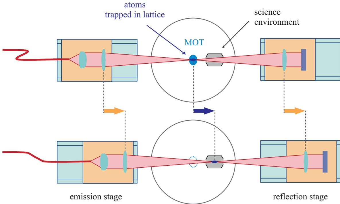
**Figure 1.** Sketch of the moving lattice setup. Atoms are loaded from the magneto-optical trap (MOT) into the lattice (upper part) and transported to the “science environment” by moving the lattice optics on both sides of the vacuum chamber with air bearing translation stages (lower part).
