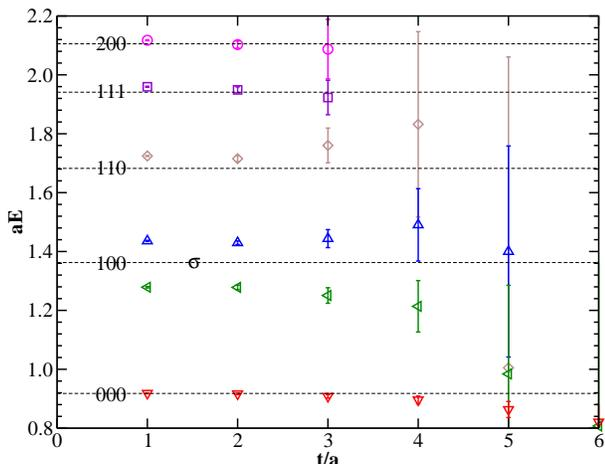
FIG. 3: Effective mass versus time as determined by the diagonalization of the correlation matrix  $C_{ij}$ . The dashed constant lines describe the free two-particle spectrum. Simulation parameters:  $\nu = 1.0$ ,  $\lambda = 1.4$ ,  $am_\pi = 0.36$ , volume= $12^3 \times 64$ .
