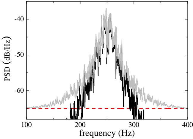
FIG. 7. **Noise spectrum.** Typical noise spectral density for  $T = 5$  ms and  $A = 1$  (black-solid line). By including the broadband background noise (red-dashed line), due to acoustic noise on the lattices' mirrors, we estimate the effective experimental spectrum (grey-solid line).
