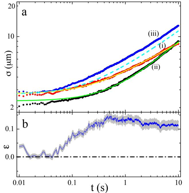
FIG. 4. **Deviations from additivity with a narrowband noise.** Numerical simulation of the time evolution of the width (a) and relative residuals (b) with the same parameters of Fig. 3c-d, but with  $T = 10$  ms. Deviations from additivity are evident in the discrepancy between the curve with noise and interaction (iii) and the solution of Eq. (3) (dashed line).
