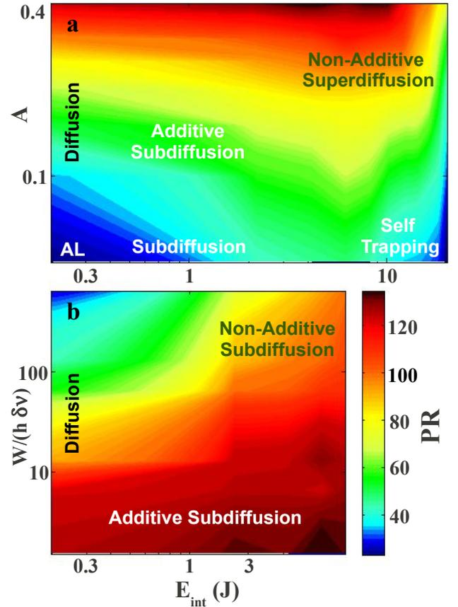
FIG. 6. **Generalized diffusion regimes.** The color scale represents the number of significantly occupied sites after 10s of our numerically simulated expansion, for  $\Delta = 2.5J$ ,  $J = 180$  Hz and a Gaussian wavepacket initially distributed over  $\approx 13$  lattice sites. a) Dependence on  $A$  and  $E_{int}$  for a broadband noise ( $\delta\nu \approx W/h$ ). b) Dependence on  $E_{int}$  and  $\delta\nu$ , for a fixed noise strength  $A = 0.4$ .
