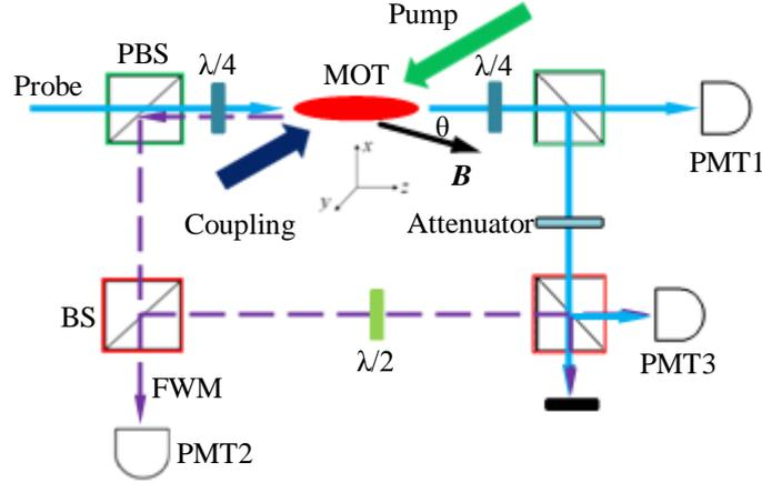
Fig. 2 (Color online) Simplified experimental setup. The photomultiplier tubes PMT1 and PMT2 (H10721, Hamamatsu) detect the signals. Meanwhile the beating of the two pulses is detected by PMT3. An attenuator is used in the probe channel to match the intensity of the two retrieved pulses so as to have a good visibility of the interference fringes.
