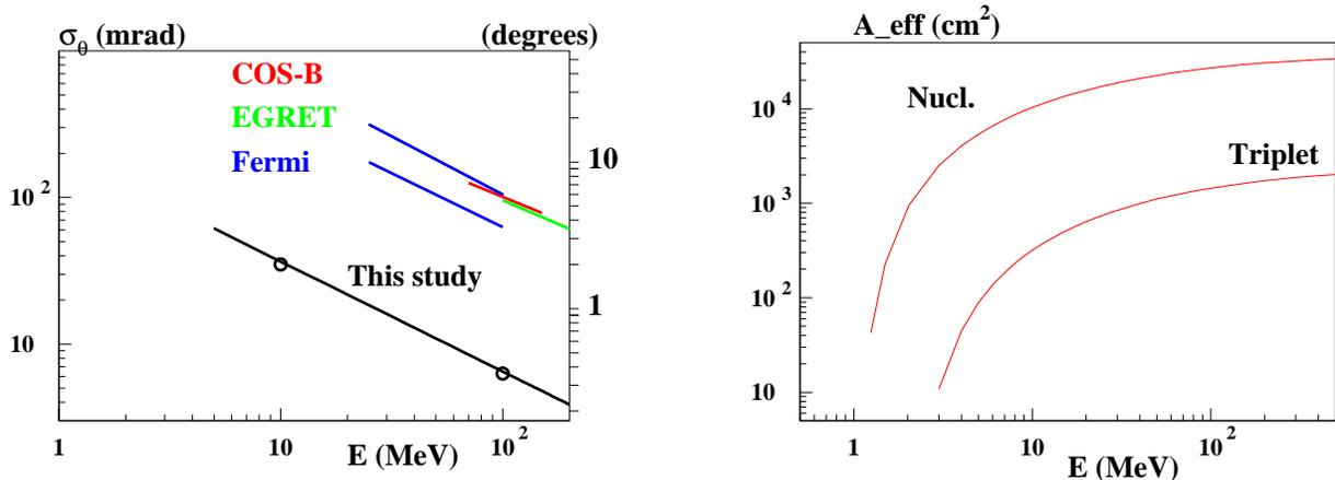
FIG. 1: Angular resolution as a function of photon energy compared to past and existing telescopes (the two *Fermi* curves correspond to “front” and “back” events, respectively). The black line is our analytical prediction while the two points are obtained from simulation (left). Effective area of a 1 ton Argon-based thin detector, as a function of photon energy, for perfect efficiency ( $\epsilon = 1$ ) (right).
