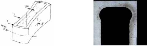
Figure 3: Schematic illustration of O-shaped crystal (left) and the microscope image of O-BNL-02 (right).
