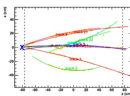
**Figure 3.** RAW and Reconstructed TPC tracks from two different events.
