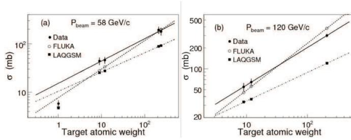
**Figure 6.** Comparison of the A-dependence of MIPP cross sections with those from Monte Carlos. The lines are fits to the data. The cross sections are for producing neutrons with momentum greater than the threshold and within an angular range of 20.4 mrad. The errors are combined statistical and systematic uncertainties. Note that the hydrogen data point is not included in the fit. The cross sections are not corrected for geometric acceptance.
