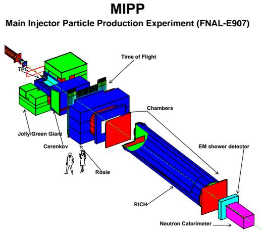
**Figure 1.** Layout of the experiment - Run I. With the MIPP upgrade we propose to add the plastic ball detector as a recoil detector surrounding the target.
