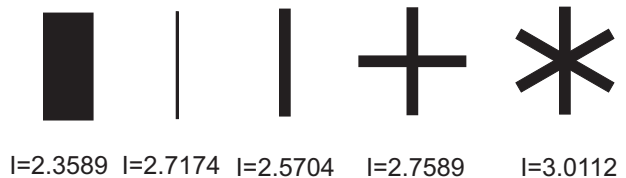
FIG. 7: The mutual information depends strongly on size and shape of the object. Here, the two objects on the left have widths 1.5w_0 and .2w_0 ; all other widths are .4w_0 .
