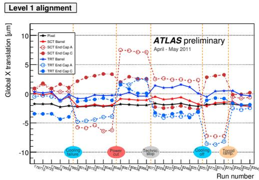
**Fig. 7.** Changes in the alignment constants on a run-by-run basis. Note the impact of incidents such as magnet ramping and cooling interruptions.
