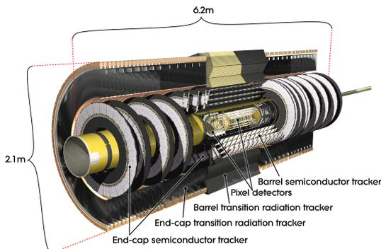
**Fig. 1.** The ATLAS Inner Detector.
