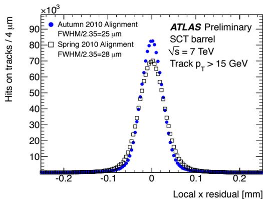
**Fig. 3.** Improvement in resolution in the direction of highest granularity of the SCT modules after the Autumn 2010 alignment.
