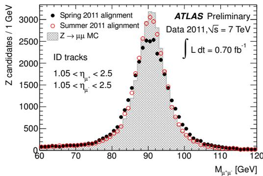
**Fig. 6.** Improvement in the Z mass resolution due to using constrained alignment to remove weak mode misalignment in the endcap A region
