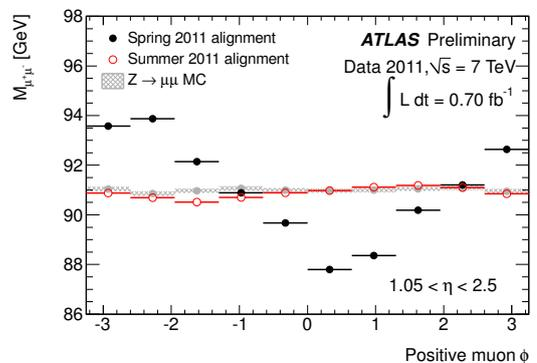
**Fig. 5.** An indication of a weak mode misalignment present in the endcap A region (black) and the effect of using constrained alignment to remove it (red).
