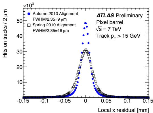
**Fig. 2.** Improvement in resolution in the direction of highest granularity of the Pixel modules after the Autumn 2010 alignment.
