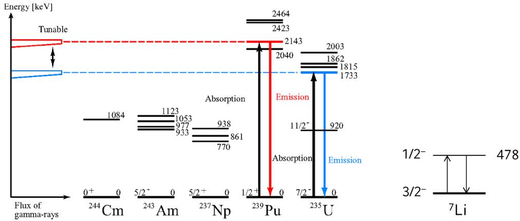
**FIGURE 3.** Nuclear resonance fluorescence M1 excitation modes in actinides.
