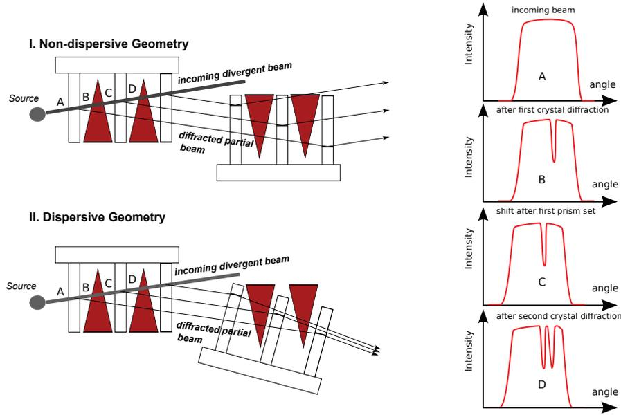
**FIGURE 1.** Schematic picture showing the successive small angular shifts between the sequence of double crystal monochromators.
