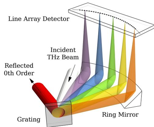
FIG. 2: Principle of the multi-channel THz and infrared spectrometer based on five stages of blazed reflection gratings in combination with focusing ring mirrors. The schematic layout is depicted in (a), and (b) shows one stage exemplarily (see Refs. [38, 39] for technical details). The fast readout of the pyroelectric detector arrays allows single-shot spectroscopy.
