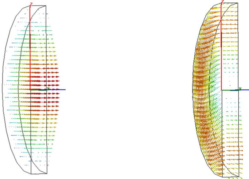
**Fig. 9:** A simple pillbox cavity, showing the electric field vector (left) and the magnetic field vector (right)
