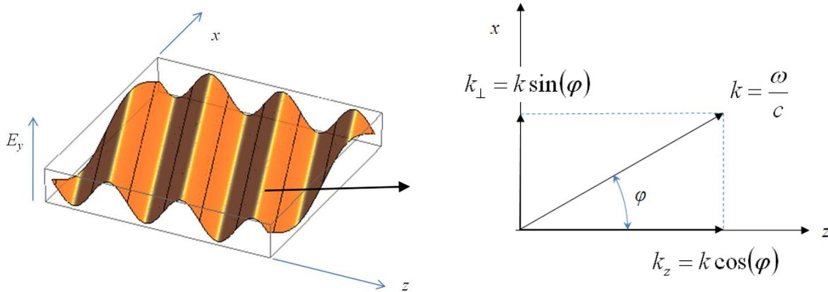
**Fig. 1:** A homogeneous plane wave, polarized in the  $y$  direction and propagating in the  $x$ - $z$  plane. Left: snapshot of the wave travelling in the direction of the arrow; right: components of the wave vector
