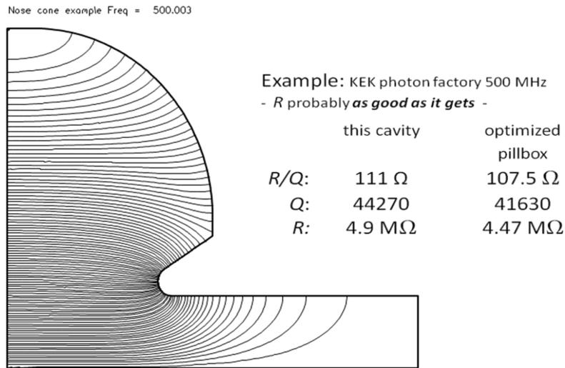
**Fig. 13:** Longitudinal section through half of a KEK photon-factory, 500 MHz, nose-cone cavity
