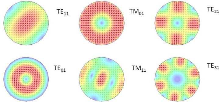
**Fig. 8:** The first six modes in a circular waveguide. The arrows of the electric fields are sketched. Modes with azimuthal index  $m \neq 0$  appear with two different polarizations, only one of which is shown
