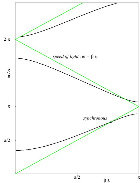
Fig. 18: A Brillouin diagram for a periodic structure
