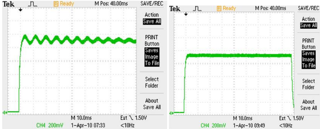
Fig. 12: Peak-detected pick-up signal showing quadrupole oscillation. Left: 8 MV. Right: 2.5 MV.
