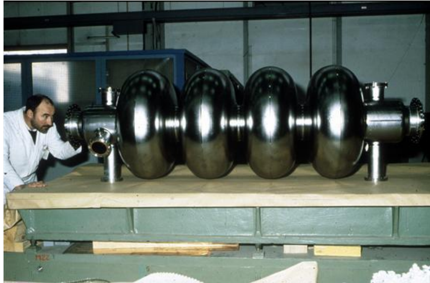
Fig. 11: 4-cell prototype superconducting RF cavity for LEP (1985)
