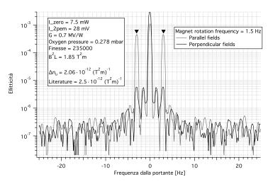
Fig. 5. Fourier spectrum around the carrier frequency  $\omega_{\mathrm{Mod}}$ . Ellipticity measurements with the magnets parallel (grey curve) and the magnets perpendicular (black curve). The large sidebands at  $2\Omega_{\rm Mag}$  are due to the Cotton Mouton effect in Oxygen gas.
