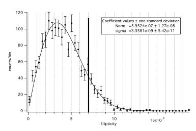
Fig. 6. Histogram of ellipticity noise in a frequency band around  $2\Omega_{\rm Mag}$ :  $(3.25\pm0.39)$  Hz. The integration time was T=8192 s. Superimposed is a fit with the Rayleigh distribution resulting in an ellipticity standard deviation  $\sigma=3.36\cdot10^{-9}$ . The vertical black line indicates the value in the ellipticity Fourier spectrum bin corresponding to  $2\Omega_{\rm Mag}=3.25$  Hz.
