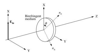
Fig. 3. Reference frame for the calculations using the Jones matrix formalism. The birefringent medium has a thicness L.
