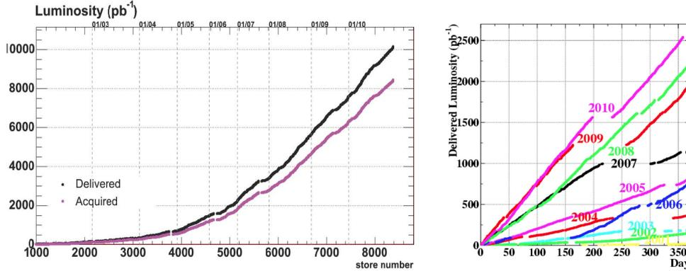
Fig. 2. Left: Integrated luminosity in Tevatron Run II as a function of time. Right: Delivered luminosity in Run II year-by-year.
