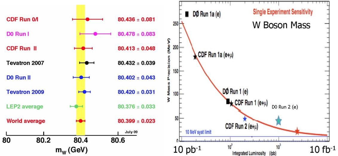
Fig. 5. W mass measurements, most recent CDF Run II result is based on 0.2/fb, while D0 Run II result is based on 1/fb. On the right side, predicted errors for W mass measurement at Tevatron.
