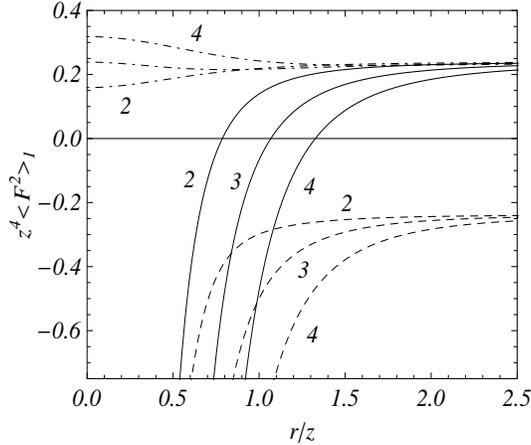
Figure 1: VEV of the field squared,  $z^4 \langle F^2 \rangle_1$ , for the electric (full curves) and magnetic (dashed curves) fields in the geometry of a single metallic plate. The numbers near curves are the values of the parameter  $q$ . The boundary-induced part in the VEV of the electric field squared is plotted separately by the dot-dashed curves.
