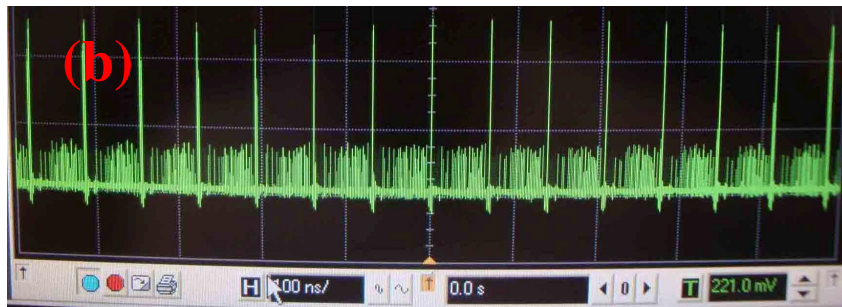
Figure 5.7: (a) Optical spectrum of dual wavelength dissipative solitons. Insert: the normalized optical spectrum; (b) Oscilloscope trace of dual wavelength dissipative solitons.
