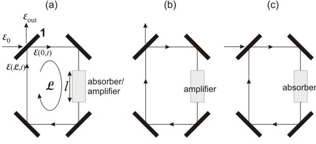
FIG. 1. (Color online) (a) Schematic of a ring cavity with a homogeneously-broadened two-level medium and an injected signal. (b) and (c) show schematically the operation of a laser and a CPA system.
