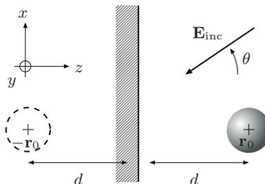
FIG. 2: Geometry of the system: A spherical dipole nanoparticle interacts with a perfect mirror. The dashed sphere corresponds to the image dipole.
