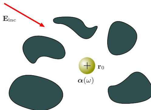
FIG. 1: Optical dipole antenna of arbitrary shape in a structured environment. A point  $\mathbf{r}_0$  inside the antenna is used to define its position.
