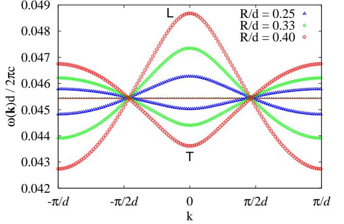
FIG. 13: (Color online) Same as Fig. 12, except that only three  $R/d$ 's are plotted, with inclusion of up to the fifth nearest-neighbors. We omit the three largest values of  $R/d$  because it may be necessary to include more than just  $\ell = 1$  when  $R/d \gtrsim 0.4$ .
