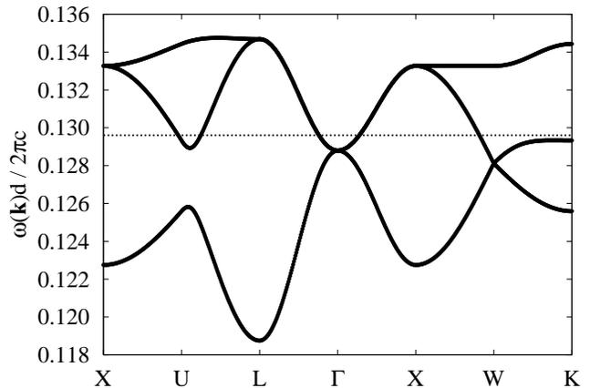
FIG. 2: Tight-binding inverse opal band structure for  $\omega < \omega_p$  with  $d = 500\sqrt{2}$  nm,  $R = 150$  nm, and  $\omega_p d/c = 1.0$ , using  $\omega_{at} d/(2\pi c) = 0.1296$  for  $\ell = 1$  in an infinite medium. The horizontal dotted line represents the “atomic” level.
