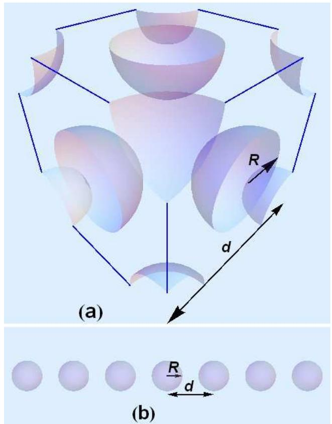
FIG. 1: (Color online) Schematic diagram for (a) an inverse opal structure with a lattice constant  $d$  and a void sphere radius  $R$ ; (b) a linear chain of nanopores with a pore separation  $d$  and a nanopore radius  $R$ .
