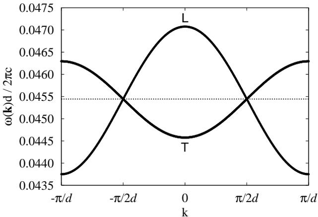
FIG. 3: Tight-binding results of a periodic chain of nanopores in a Drude metal host, for  $\omega < \omega_p$ . We use  $d = 75$  nm,  $R = 25$  nm, and  $\omega_p d/c = 0.35$ , using  $\omega_{at} d/(2\pi c) = 0.0454$  for  $\ell = 1$  in an infinite medium. Only the nearest-neighbors are included. The horizontal dotted line represents the “atomic” level. In this and the following all plots, “L” and “T” denote the longitudinal and transverse branches, respectively.
