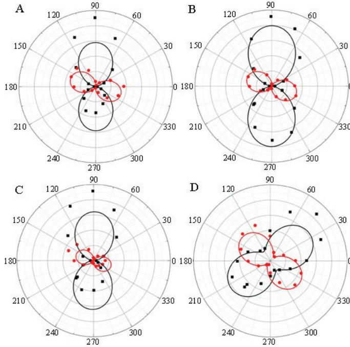
Figure 3: Measured polarisation data for NVs A, B, C and D. The radius represents the emission intensity and the angle is that of the polarizing filter,  $\phi_p$ . The solid curves are fits to the function  $I_0 + \Delta I \cos^2(\phi_p + \phi')$  where  $I_0$ ,  $\Delta I$ , and  $\phi'$  are fitting parameters.
