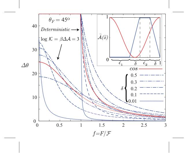
FIG. 2. Effect of  $\delta$  on the deflection angle as function of the normalized force in the stochastic and deterministic regimes. The solid lines correspond to the cosine potential while the dashed lines correspond to the LTD potential for different transition regions and  $\epsilon_1 = \epsilon_2 = 0.5 - \delta$ . The curves corresponding to the Brownian case and the respective deterministic curves have the same line style. The inset shows schematics of the cosine and the LTD potentials.
