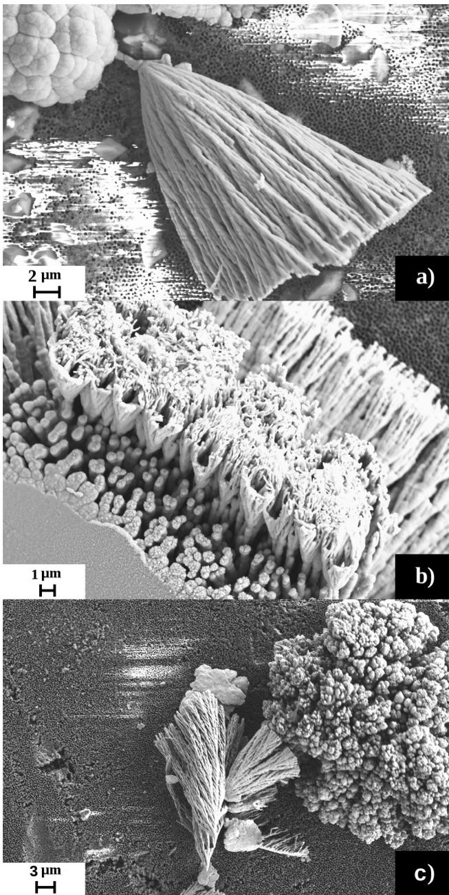
**Figure 2.** Volume PdNi alloy structures on the membrane surface: a) “faded algae”, b) structures at different stages of growth, c) “twisted algae” and “cauliflower” formed nearby.
