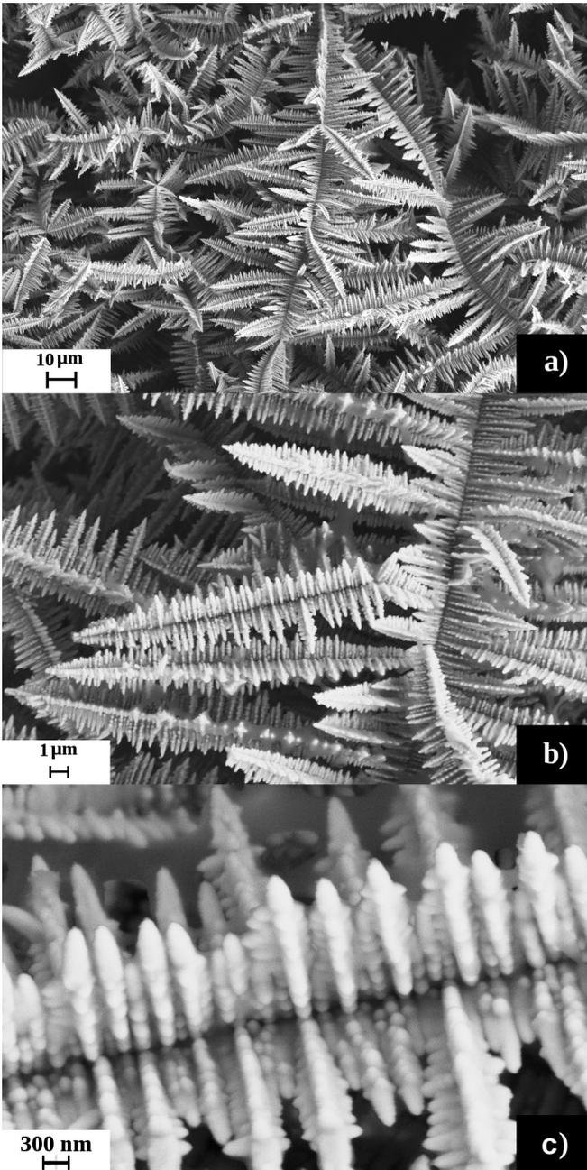
**Figure 7.** “Fern” formed by alternate electroplating of PbIn and PdNi alloys. a) general view b), fern “leaves” c), “fern stem”
