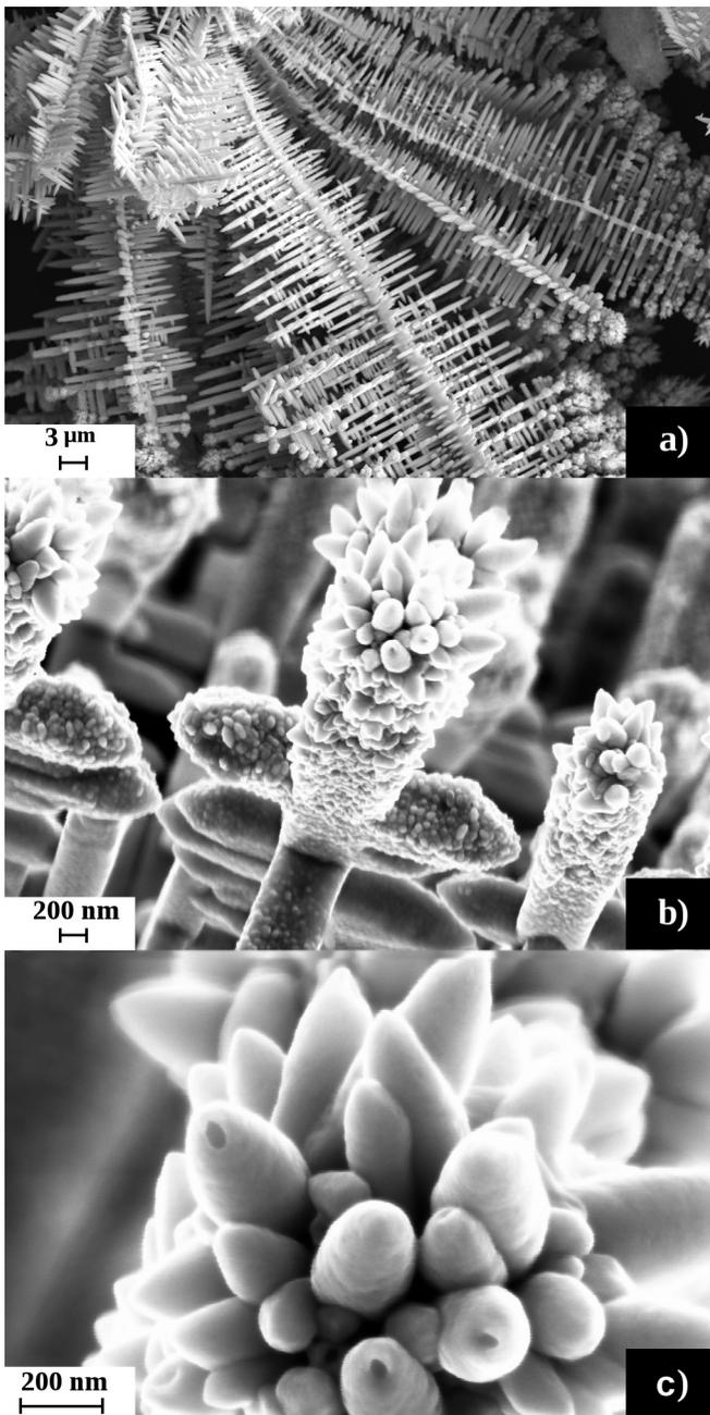
**Figure 8.** “Flower wreath” formed by alternate electroplating of Pb and PdNi alloys. a) general view of the structure, b) a single “leaf”, c) a single “bud”.
