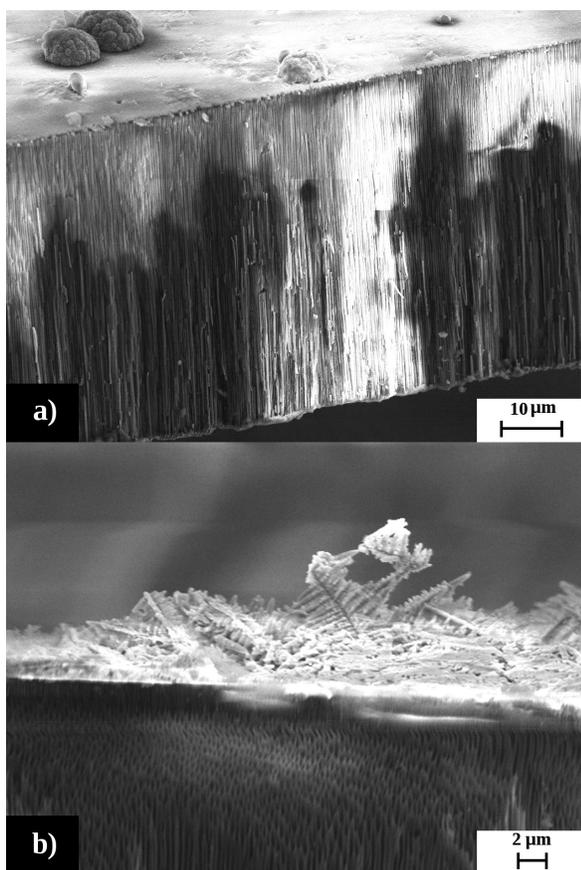
**Figure 1.** Cross section of the membrane with nanowires inside and structures on the surface a) PdNi alloy “cauliflower”, b) PbIn and PdNi alloy “fern”.
