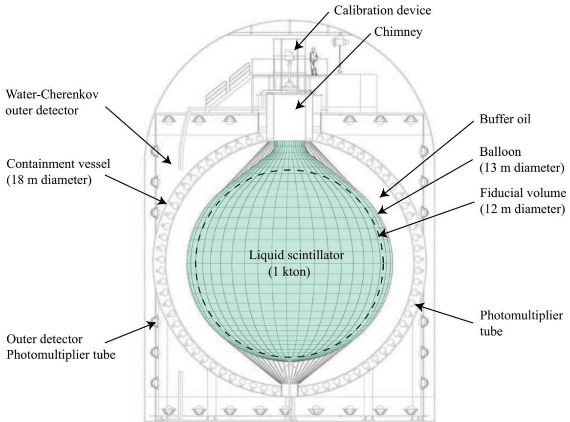
Fig. 1.— Schematic diagram of the KamLAND detector.
