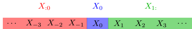
FIG. 3. A process’s time series: Time indices less than zero refer to the past X_{:0} ; index 0 to the present X_0 ; and times after 0 to the future X_{1:} .
