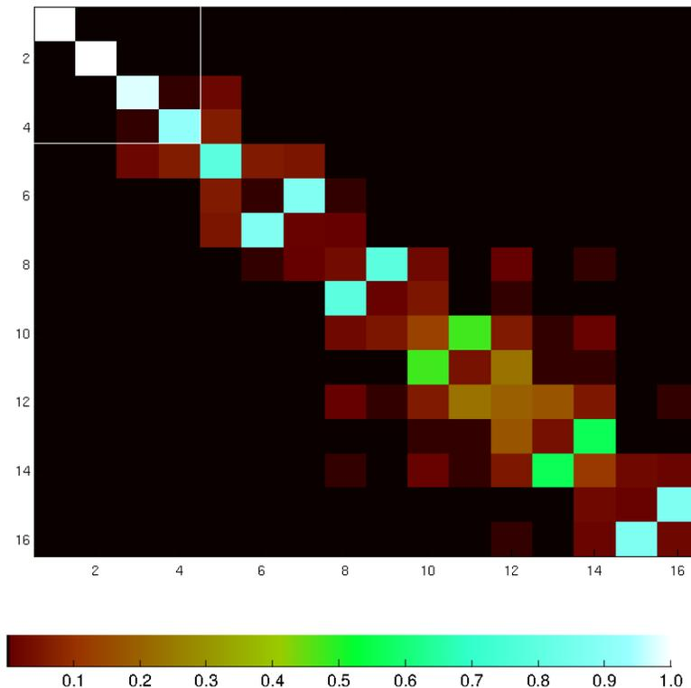
Figure 4: (color online) Entanglement map for the  $L=-1$  sector ground state (note that this is not the global ground state) for a Majumdar-Ghosh chain of 16 spins with 4 adjacent spins, whose position is indicated by the white square, subjected to a local magnetic field of strength  $h=5J$ . The color scale is normalized to 1 as shown.
