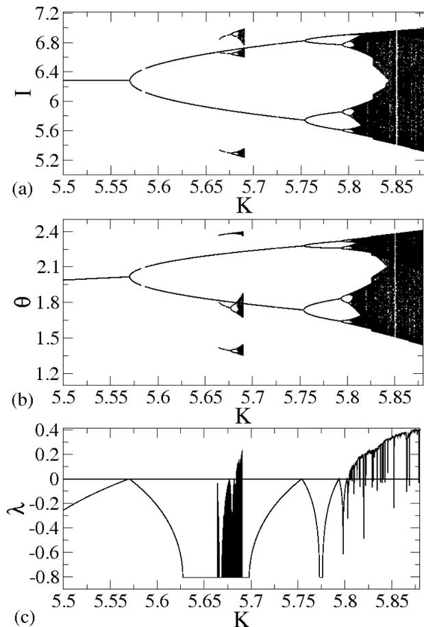
FIG. 1: Bifurcation cascade for (a)  $I$  and (b)  $\theta$  both plotted against the parameter  $K$ . In (c) it is shown the Lyapunov exponent associated to (a) and (b). The damping coefficients used for the construction of the figures (a), (b) and (c) were  $\gamma = 0.80$ .
