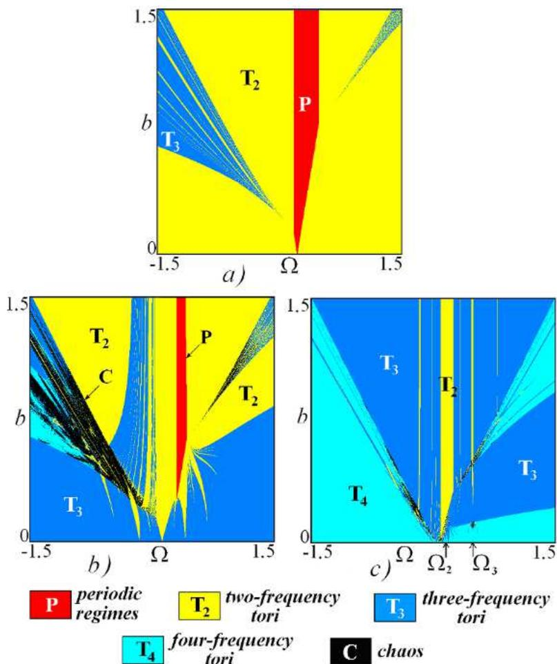
Figure 2: Charts of Lyapunov exponents for the model systems of two (a) and three (b and c) driven oscillators. Parameter values are  $\Delta_1 = 0.3$ ,  $\Delta_2 = 1$ ,  $\mu = 0.4$  (a),  $\mu = 0.4$  (b),  $\mu = 0.15$  (c). The color coding is indicated in the bottom part of the figure. The marks  $\Omega_2$  and  $\Omega_3$  indicate frequencies of the second and the third oscillators respectively.
