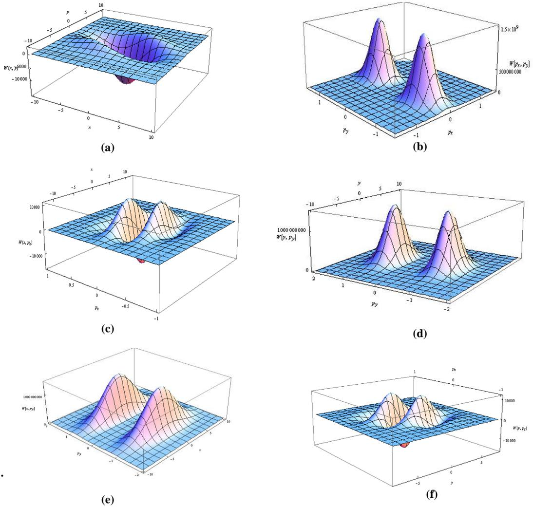
**FIGURE 1.** Plot of Wigner function (in arbitrary units) for  $m = 3$ , with  $\sigma_x = 5$ ,  $\sigma_y = 3$  as a function of (a)  $x$  and  $y$  (b)  $p_x$  and  $p_y$  (c)  $x$  and  $p_x$  (d)  $y$  and  $p_y$  (e)  $x$  and  $p_y$  (f)  $p_x$  and  $y$  [14].
