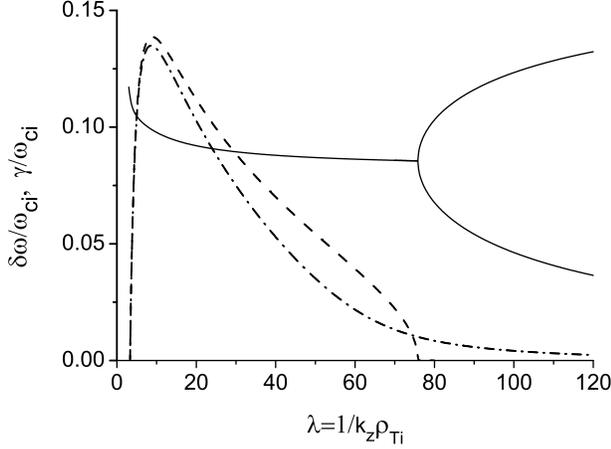
Figure 1: The dispersion (solid line) and the growth rate (dashed and dashed-dotted lines) of the EIC oscillations versus the normalized wavenumber. Dashed line - the growth rate with neglecting the Landau damping by electrons, dashed-dotted line - the growth rate accounted for the Landau damping by electrons.  $S_i = 3, k_{\perp} \rho_{Ti} = 1$ .
