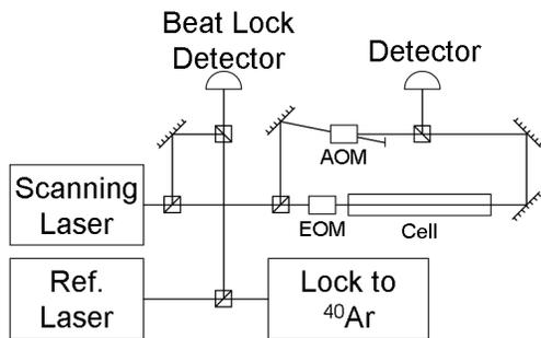
FIG. 2: A schematic of the saturated absorption spectroscopy setup. The 1 m long spectroscopy quartz cell is filled with a mixture of an enriched  $^{39}\text{Ar}$  sample ( $^{39}\text{Ar}/^{40}\text{Ar} \sim 1.5 \times 10^{-3}$ ,  $\sim 0.5$  Torr partial pressure) and natural krypton ( $\sim 2$  mTorr partial pressure).
