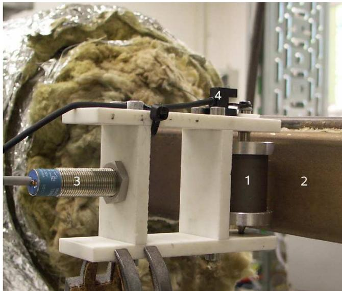
Figure 5: Single-magnet rotary flowmeter with a *SmCo*-type magnet (1) of 24 mm and 35 mm in diameter and height, respectively, installed at the side of a rectangular stainless steel duct (2) of  $45 \times 45 \text{ mm}^2$  in cross-section carrying the liquid sodium flow. The rotation rate is measured with an inductive magnetic proximity sensor (3) and also monitored with a photoelectric barrier sensor (4).
