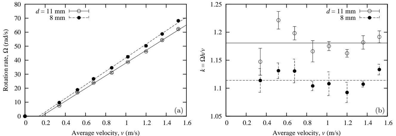
Figure 6: Measured (a) and rescaled (b) magnet rotation rates along with the best linear fits versus the average velocity for  $d = 8$  mm and 11 mm gaps between the magnet and the duct with the distance between the magnet axis and liquid metal  $h = R + d_w + d$ , where  $R = 12$  mm is the magnet radius and  $d_w = 3$  mm is the thickness of stainless steel wall.
