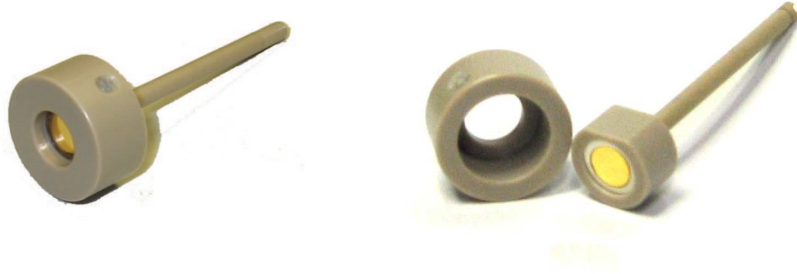
Figure 4: Photo of the proton source assembled (left) and disassembled (right). The gold-colored disc is the americium. The cylindrical cap holds the mylar foil.
